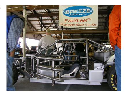
Now that we have completed the chassis design with opening doors, we will be moving on to the design of the body mounting structure and crush panels. Our goal is to develop a body and body mounting kit that minimizes or even eliminates the need for custom fabrication. We will also be specifying the fuel system, brakes, shocks, cooling system and rear-end, seats, dash and gauges and exhaust systems, most of which will drop ship directly from the race-car parts manufacturer to the customer.
